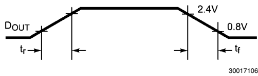
FIGURE 4. D OUT Rise and Fall Times
